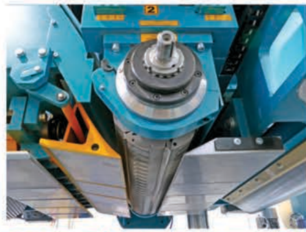
Bottom and top cutter shaft for 1000 and 1300 mm wide planers.
