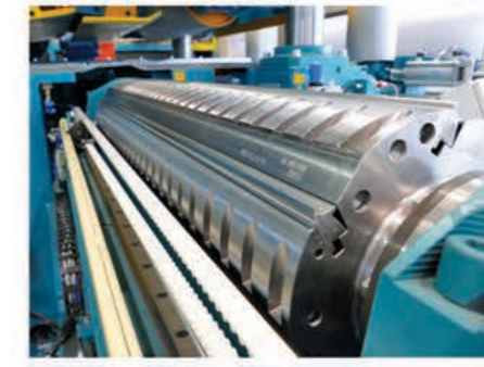
Cutter shaft of 2300 and 2600 mm wide planer.
