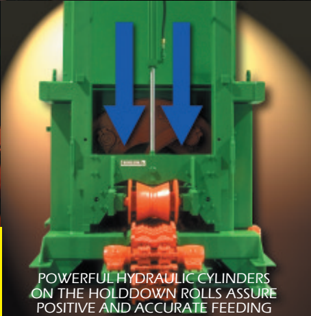
DEBARKER RING MOVES UP AND DOWN TO CENTER ON THE INCOMING LOG
